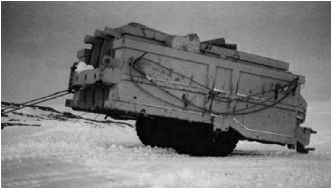
a. Towed compaction roller used at Molodezhnaya. These pneumatic-tire rollers are ballasted with concrete, some to 17.2 tonne and one to 30 tonne. Each pulls a simple drag. (Photo by M. Mellor, 15 November 1990.)
