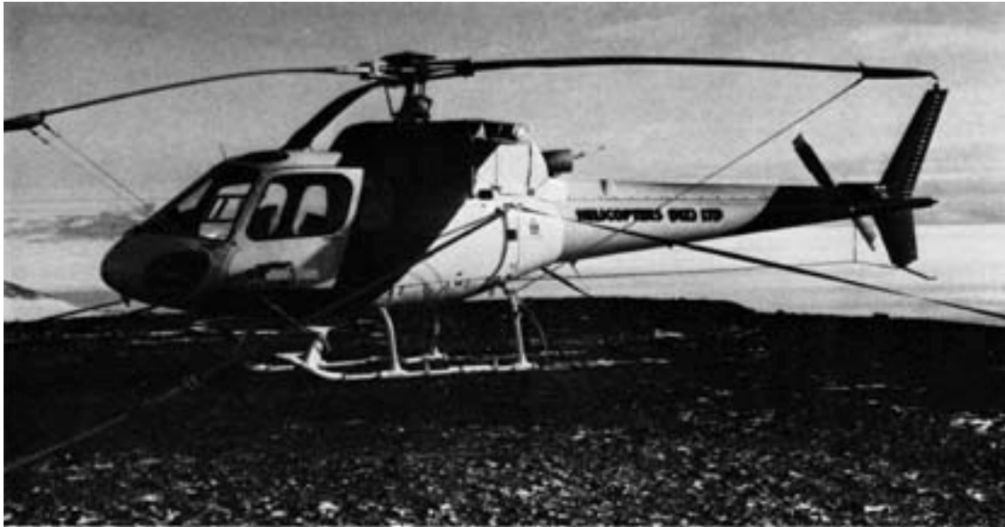
e. Aerospatiale AS350 Ecureil, or Squirrel. This is the helicopter currently favored for Antarctic operations by Australian and New Zealand contractors. It has a bit more power and lift (and higher fuel consumption) than the 206. (Photo by M. Mellor, October 1990.)
