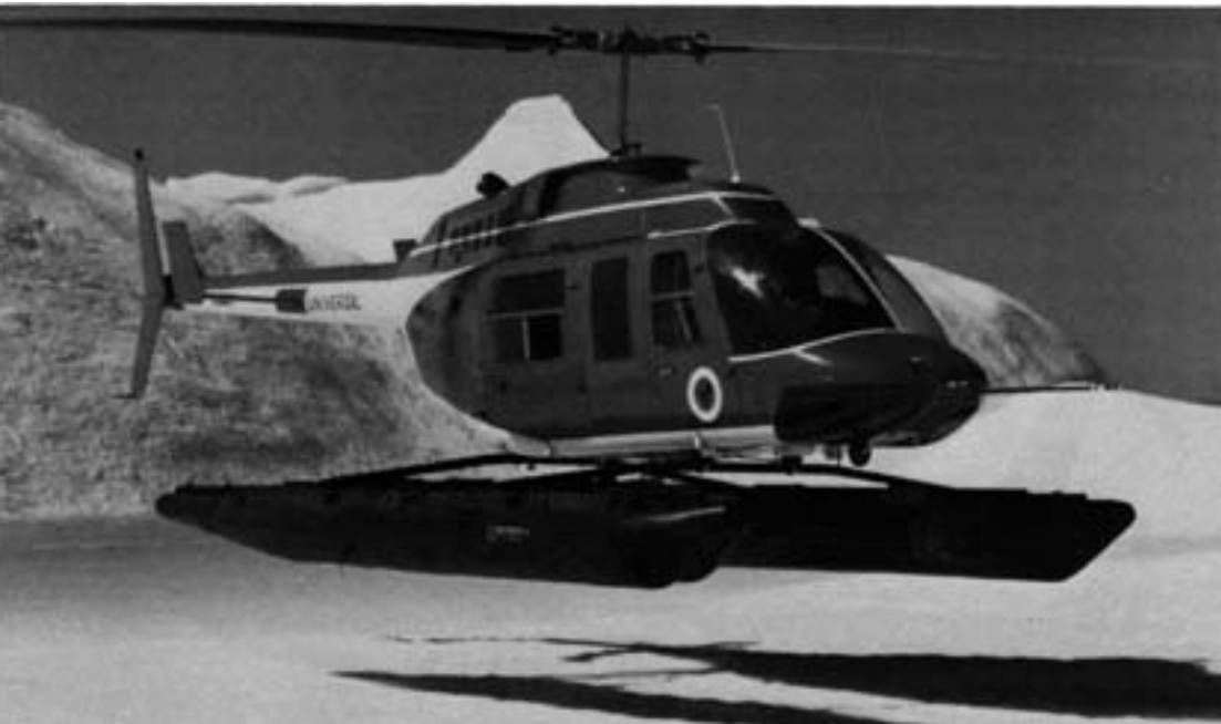
d. Bell 206 (Jet Ranger) on floats. Although much less powerful than the 212, it can handle a wide range of science support tasks. (Photo by M. Mellor, August 1984.)
