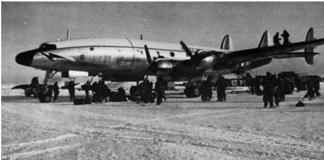
Figure 15. USN Lockheed Super Constellation (C-121J or R7V) on the sea ice at McMurdo. The Super Constellation (first flown in October 1950) was a derivative of the original C-69 Constellation (first flown in January 1943). It had an MTW of 156,000 lb and four 3400-hp Wright turbo-compound radials. It carried passengers between Christchurch and McMurdo in backward-facing seats, with enough room to change clothes in mid-journey. The cruise speed was 280 knots. The C-121 was the last piston-engine aircraft used by the USAP, being phased out at the end of 1970. An EC-121 (WV-2) magnetometer aircraft landed short and was destroyed at McMurdo in October 1960. In October 1970, C-121J Pegasus crashed while landing below minimums on the glacier-ice runway at Outer Williams Field. (Photo by M. Mellor, October 1961.)
