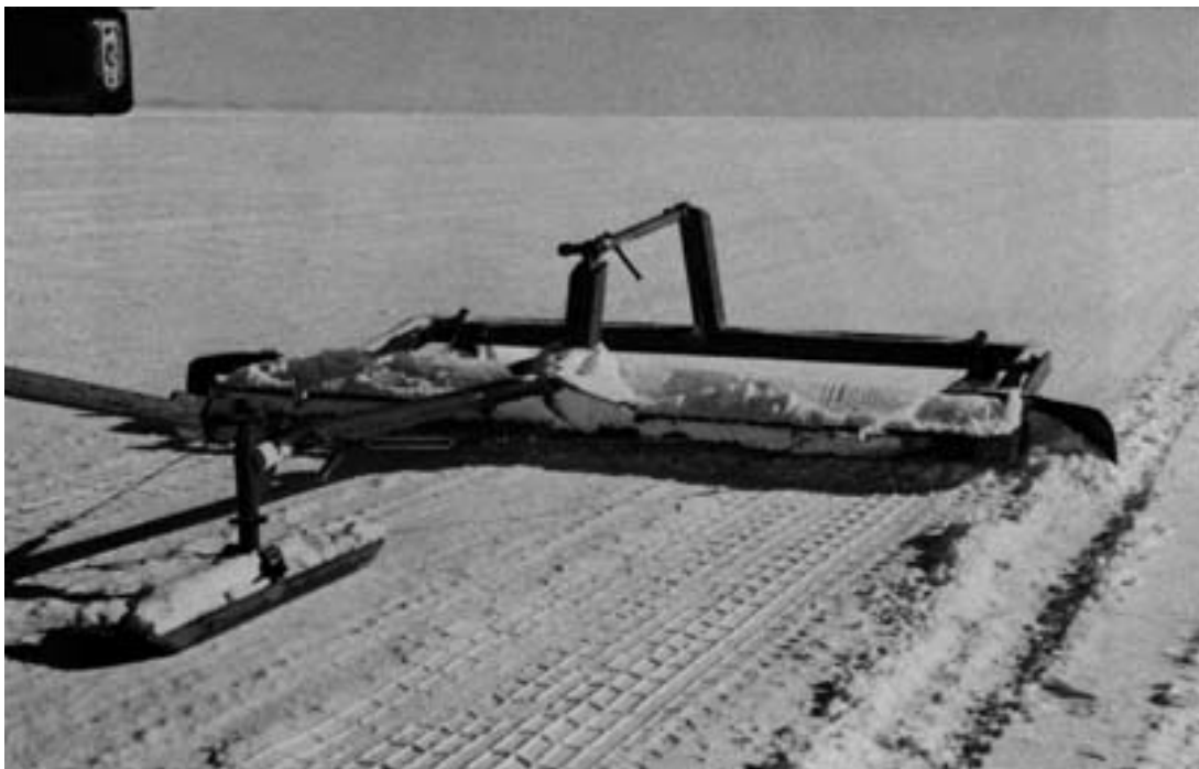
Figure 54. Small articulated drag for grooming snow roads and skiways. (Photo by M. Mellor, January 1991.)
