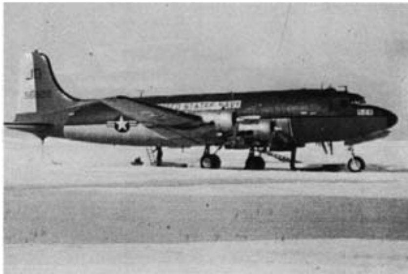
Figure 12. USN Douglas R5D (DC-4 Skymaster, or C-54) at McMurdo. The USAF also flew C-54s to McMurdo until about 1963. These aircraft operated on standard wheels between Christchurch and McMurdo. The DC-4 (prototype first flown in June 1938, production model first flown in February 1942) had an MTW of 73,000 lb, with four 1450-hp P&W radials. Altogether 1242 were built. (Photo by M. Mellor, November 1962.)
