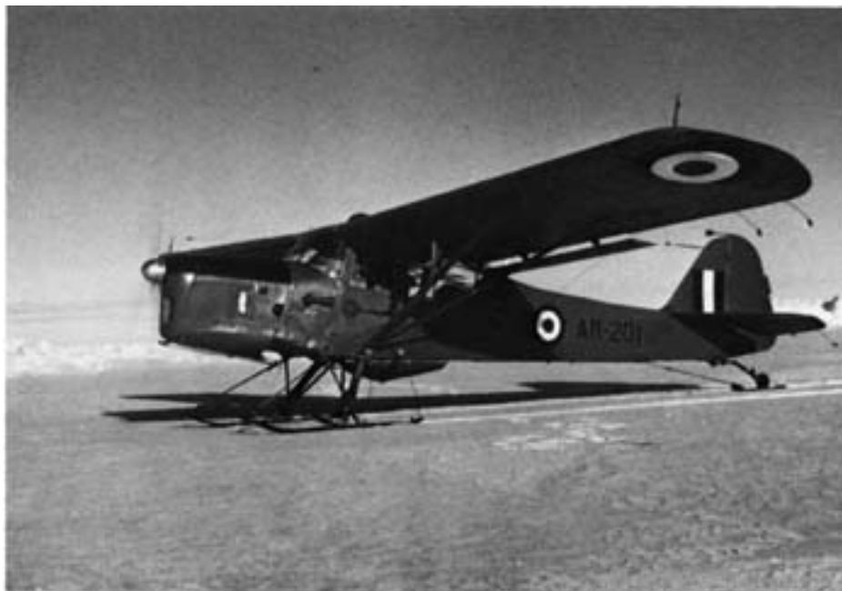
Figure 9. ANARE Auster (AOP Series, Mark 6, 145 hp DH Gypsy Major 7) on the pack ice north of Mawson. A descendant of the U.S. Taylorcraft, this model had a nominal MTW of 1990 lb (900 kg) and an actual Antarctic MTW of 2200–2400 lb (1000–1100 kg). The Antarctic variant had nonstandard oleo legs. Two of these aircraft joined the RAF as VX126 and VX127. They flew with the Norwegian–British–Swedish expedition in 1950 before transferring to the RAAF Antarctic Flight as A11-200 and A11-201 for the establishment of Mawson (1954). A11-200 was pushed overboard from Kista Dan during a storm in March 1954. After a rest with the Royal Victorian Aero Club, A11-201 rejoined the RAAF for residence at Mawson (1956–1958). It made a final trip south on floats aboard Magga Dan in 1959 for the Wilkes takeover. (Photo by M. Mellor, August 1957.)
