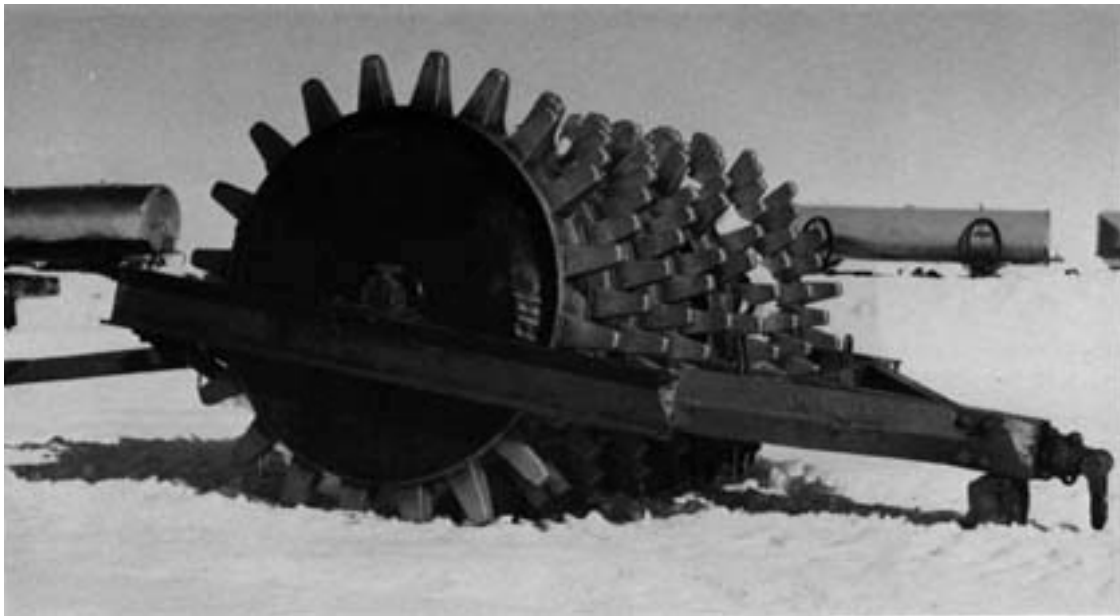
c. Sheepfoot roller, which puts high pressure on its teeth, penetrating the snow and achieving compaction at some depth below the surface. It destroys the surface layer in the process. (Photo by M. Mellor, January 1991.)
