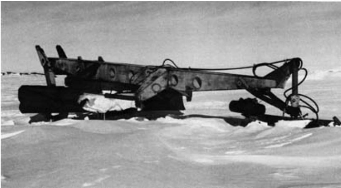
f. Ski-mounted towed grader used by the Soviet Antarctic Expedition. (Photo by M. Mellor, 15 November 1990.)
