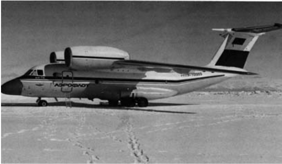
Figure 29. Antonov An-74 (MTW 76,000 lb; two Lotarev turbofans) of the Soviet Antarctic Expedition. The An-74 was developed from the An-72 (first flown in December 1977), specifically for polar operations (according to a Soviet colleague, “it is an An-72 painted red”). SSSR-72003 made the first wheel landing and takeoff on compacted snow in the high interior of Antarctica, at Vostok in November 1988. This white-knuckle feat has not been repeated so far. The aeroplane made ruts 20–30 cm deep and finally got off on the third try. (Photo by M. Mellor, 27 November 1988.)
