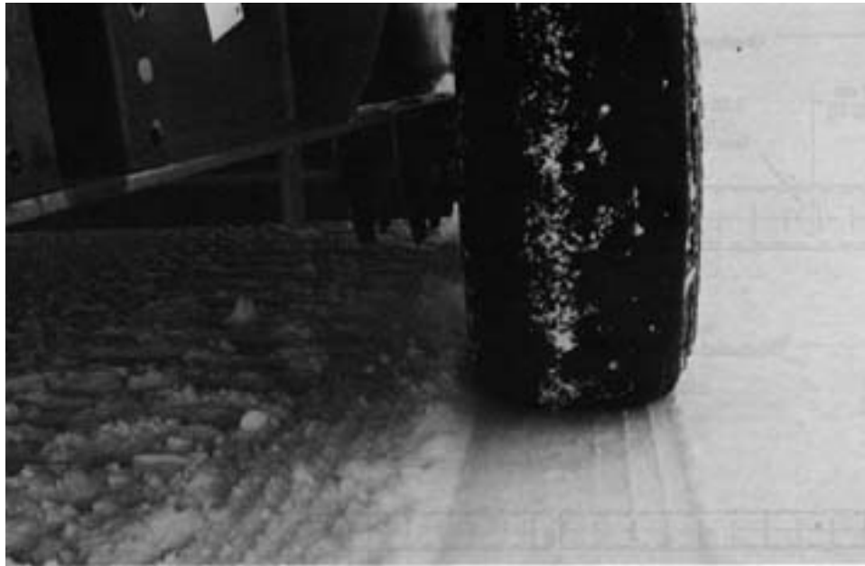
Figure 60. Imprint made in the snow runway by C-130 wheels on the Casey test cart. (Photo by Bob Sheers, Australian Antarctic Division, February 1990.)
