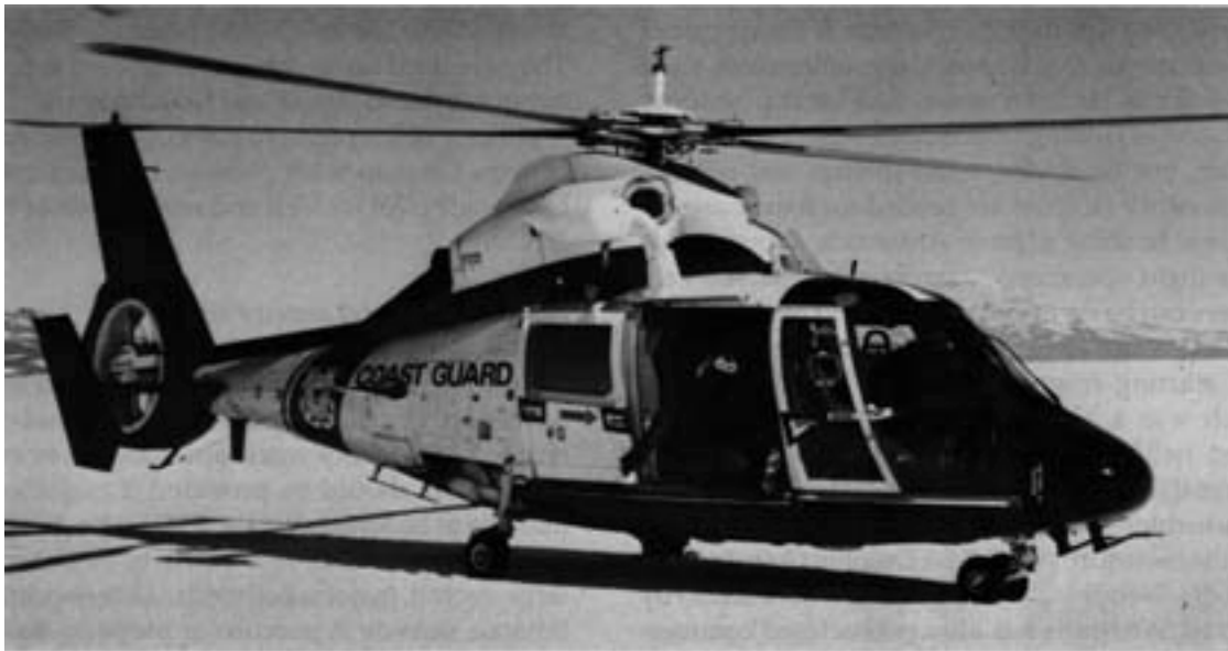
f. Aerospatiale SA366G Dauphin, or HH65A Dolphin. Dolphins are carried by USCG icebreakers in Antarctica. (Photo by M. Mellor, 29 January 1991.)
