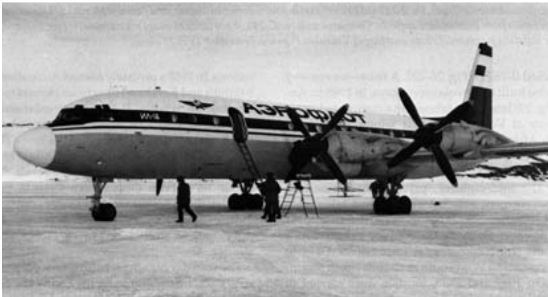
Figure 25. Ilyushin Il-18D of the Soviet Antarctic Expedition (MTW 141,000 lb; four 4250-hp Ivchenko turboprops). Chartered from Aeroflot and flown by an Aeroflot crew, the Il-18D carries passengers and light cargo between Maputo (Mozambique) and Molodezhnaya. This machine (SSSR 74267) has an extended tail cone (like the anti-submarine version) for magnetic and gravity surveys in Antarctica; it was used originally by Mr. Kosygin when he was Prime Minister. With a cheerful flight deck, quiet cabin, comfortable seats and two stewards, it is an aircraft of choice for the Antarctic frequent flyer. Contrary to popular legend, it seems unlikely that the Il-18 (first flown in July 1957) was copied from the smaller Lockheed Electra (first flown in December 1957), which was a flop until its 1979 rebirth as the P-3 Orion. Both were probably inspired by the larger Bristol Britannia (first flown in August 1952), the last aeroplane to provide real transatlantic comfort. (Photo by M. Mellor, 15 November 1990.)
