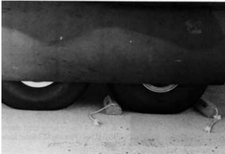
Figure 40. Wheels of the C-130. The four main wheels (56 × 20.0) are usually inflated to 96 lbf/in. 2 for operation at high takeoff weight (e.g. 155,000 lb). This gives a normal tire deflection of 32%. For operation from unpaved airstrips, the inflation pressure can be reduced until the maximum permissible deflection of 39% is reached, at which stage the tire contact area has increased to 28% above normal. At high takeoff weight (e.g. 155,00 lb) the lowest permissible inflation pressure is 75 lbf/in. 2 With a gross weight of 100,000 lb, the inflation pressure can be reduced to 45 lbf/in. 2 The nose gear (39 × 13) inflation pressure stays the same at 60 lbf/in. 2 (Photo by M. Mellor, December 1988.)
