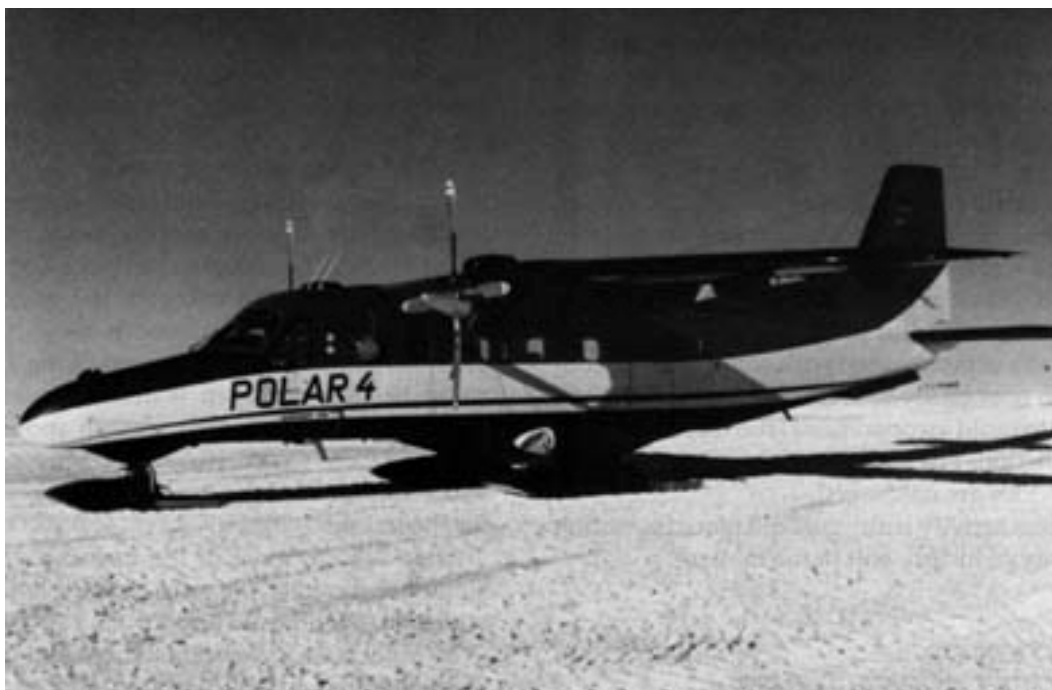
Figure 33. Ski-wheel Dornier 228-100 of the German Antarctic Expedition at South Pole Station. The Dornier 228 (first flown in March 1981; MTW 12,600 lb; two 715-hp Garrett turboprops) serves similar purposes to those of the Twin Otter; it is faster (maximum cruising speed of 231 knots at 10,000 ft, 199 knots at sea level), but it needs a bit more room for taking off and landing. (Photo by W. Tobiasson, January 1990.)
