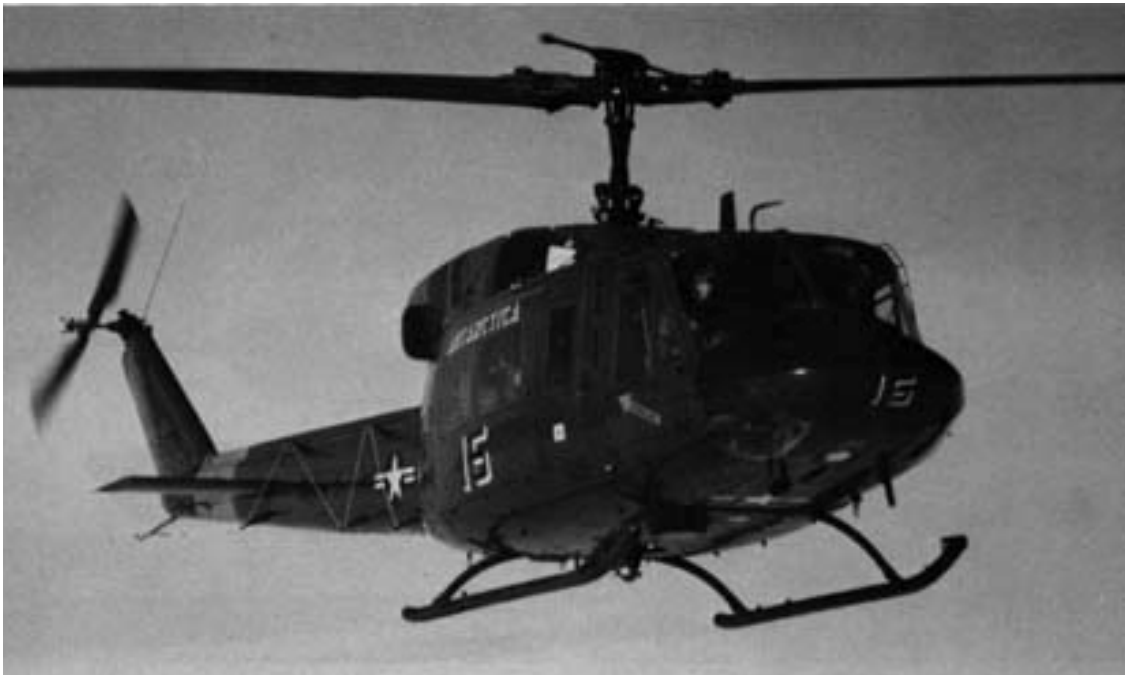
b. Bell 212 (UH-1N) helicopter. The 212 is a twin-engine machine that evolved from the single-engine 204, or UH-1. (Photo by M. Mellor, November 1990.)
