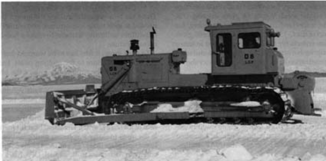
Figure 66. Caterpillar LGP-D8 bulldozer used for scraping hard snow from the surface of glacier ice in airfield construction experiments. This ancient machine was built in 1956, but for planing ice surfaces it is better than modern machines because of its long tracks. The ground contact length is 160 in., or 4.1 m. (Photo by M. Mellor, January 1991.)
