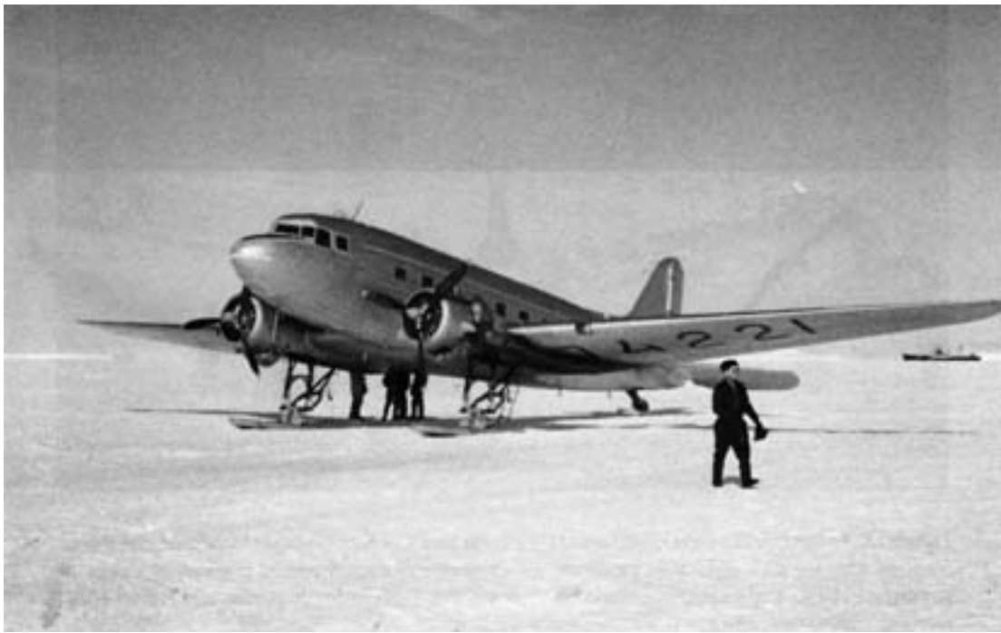
Figure 11. Lisunov Li-2 on skis (no mainwheels) near Mirny. In 1939 the U.S.S.R. began to build the Douglas DC-3 under license, first using the designation PS-84 and later redesignating the aircraft Li-2 (apparently for B.P. Lisunov, who seems to have added a window aft of the pilot's side window). Widely used in WWII, it was powered by two Shvetsov 1000-hp radials. The DC-3 and the Li-2 were the last of the big tail-draggers in Antarctica. (Photo by Charles Swithinbank, 19 January 1964.)
