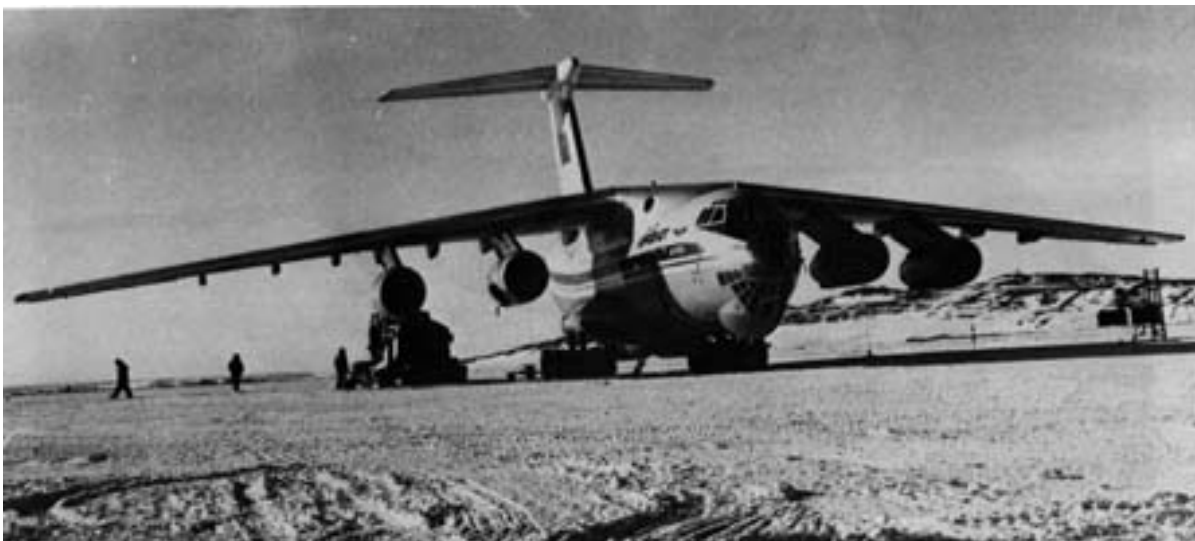
Figure 28. Front view of the Ilyushin Il-76TD at Molodezhnaya. Like the C-141 the wing has anhedral. The wing tip clearance is greater than that of the C-141—about 15.6 ft (4.74 m) unloaded. The aeroplane is powered by four Soloviev turboprops, each rated at 26,500 lbf of thrust (30% more than the C-141). The width of the mainwheel assembly can be seen on the starboard side (the MLG and nose gear have twice as many wheels as the C-141). This particular aircraft has been modified for Antarctic service with passenger seating, soundproofing, galley and in-flight working area. (Photograph by Vladimir Nazarov, November 1990.)
