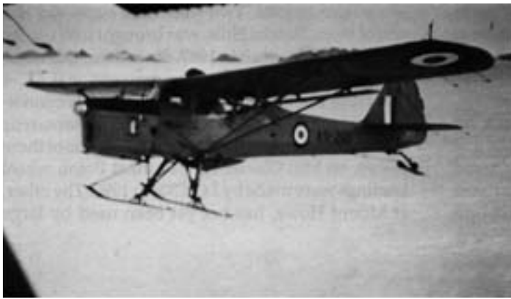
Figure 35. Simple skis, which save weight and drag and are satisfactory for small aircraft operating only on snow and ice. The Angry Ant had skis, ski-wheels and floats. It had a shotgun-cartridge starter, could run on mogas and could fly backwards in a strong katabatic wind. (Photo by M. Mellor, August 1957.)
