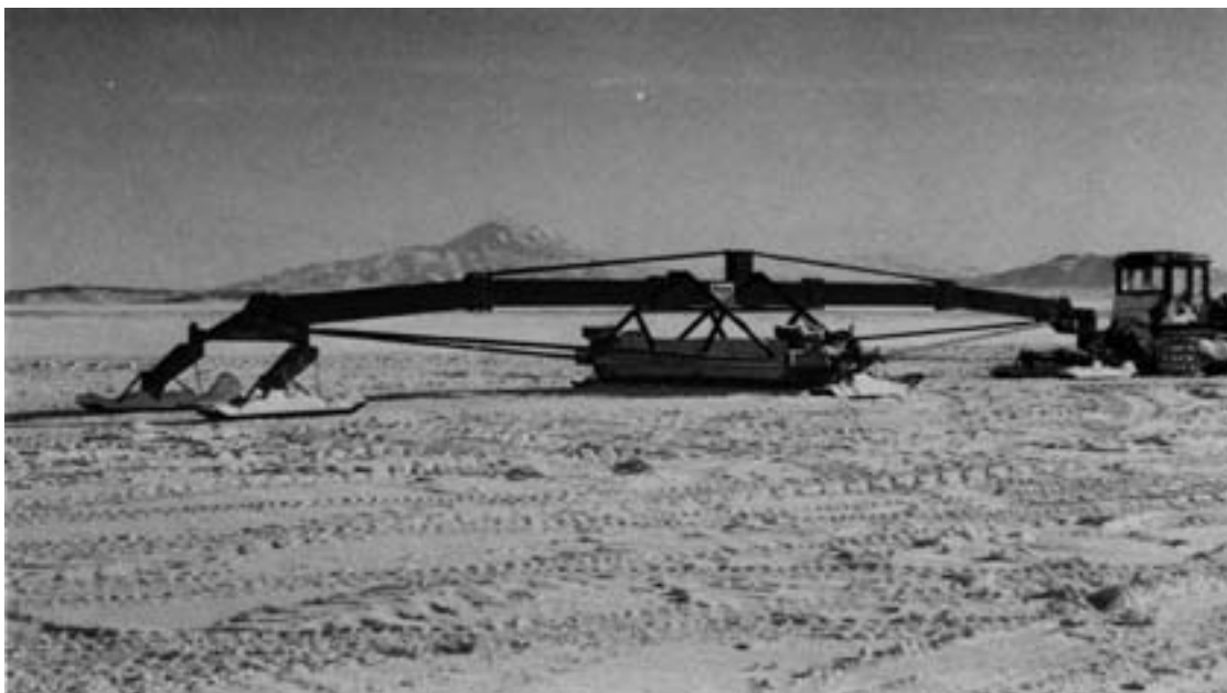
d. "Automatic" snowplane, on which the cutting depth of the moldboard is adjusted through mechanical linkages by relative vertical motion in the skis. The blade height is adjusted hydraulically by the tractor driver, so that only one operator is required. More sophisticated automatic levelers were developed by CRREL (Abele 1990), but they were heavy, expensive and perhaps a bit too complicated for reliable operation in polar service. (Photo by M. Mellor, November 1990.)
