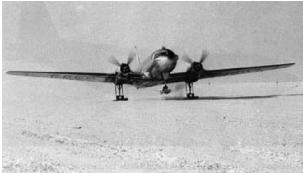
b. Piston-engine takeoff run, with the nose high and apparently no flaps. Attachment of skis to the main gear can just be made out.
