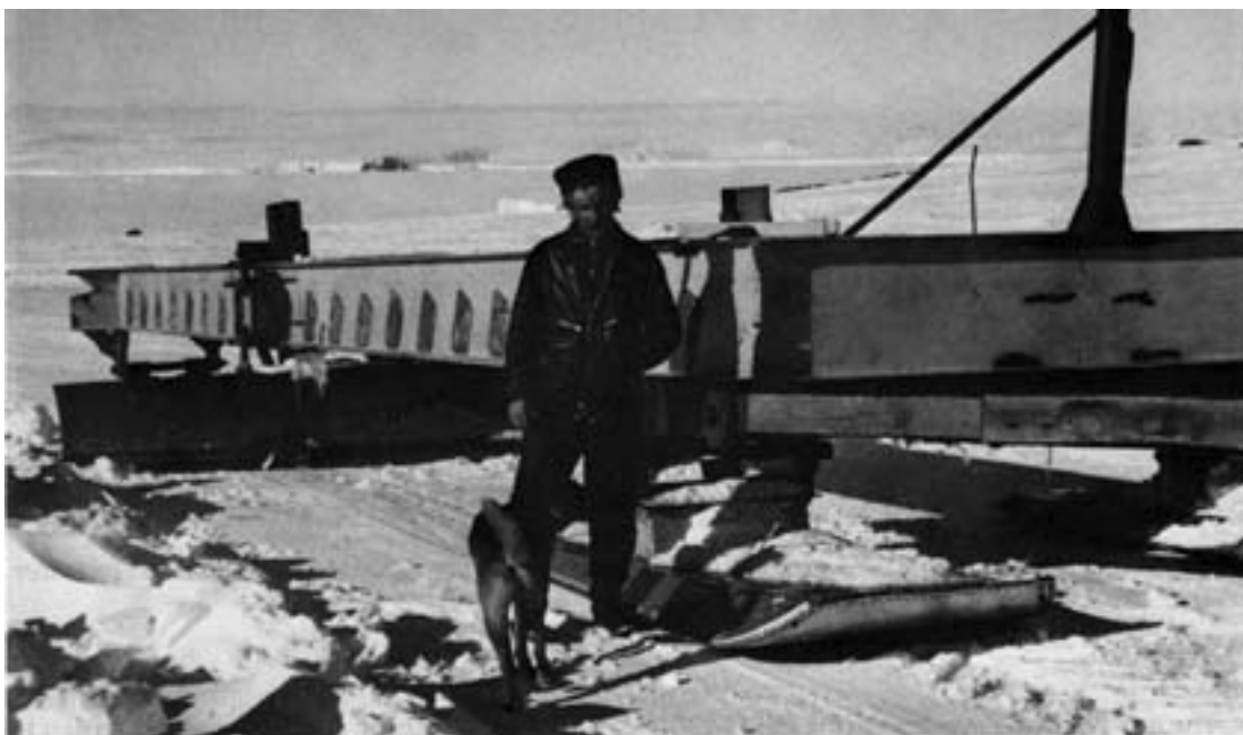
e. Ski-mounted grading plane used at the Molodezhnaya snow runway. The device operates with a fixed blade setting. The skis are the type used on An-2 aircraft. (Photo by M. Mellor, 15 November 1990.)
